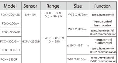
Temp./humi. range can be changed to  $-55.0^{\circ}$  C  $\sim 99.9$  C / 10 $\sim 95\%$
