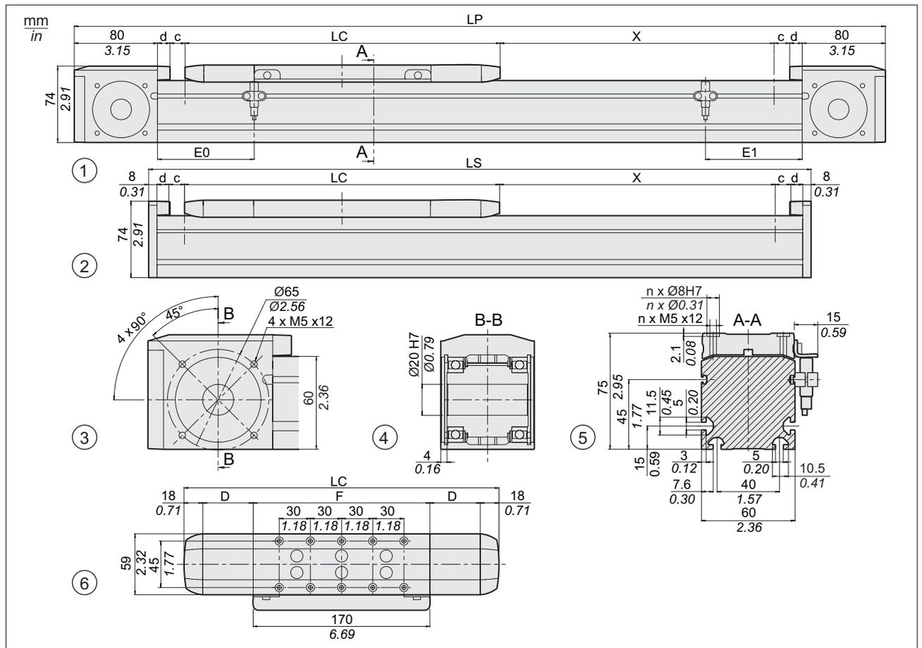
Figure 36: Dimensional drawings PAS42B
