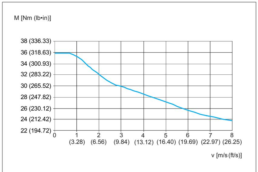
Figure 41: PAS43BR Maximum driving torque  $M_{max}$
