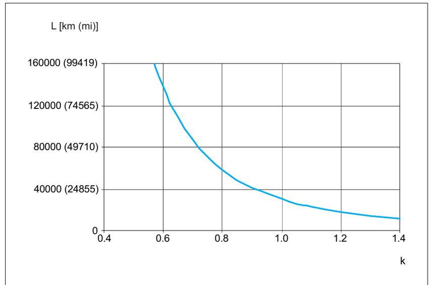
Figure 45: PAS43BR Service life load curve
