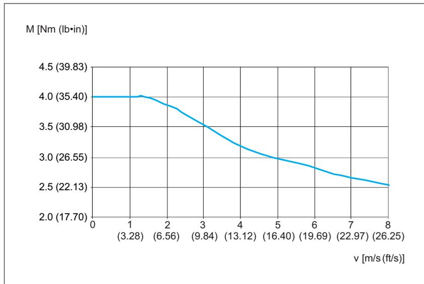
Figure 10: PAS41BR Maximum driving torque  $M_{max}$
