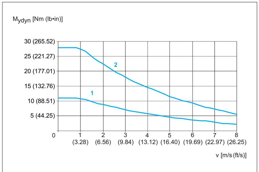
Figure 12: PAS41BR Maximum torque carriage  $M_{ydyn}$
