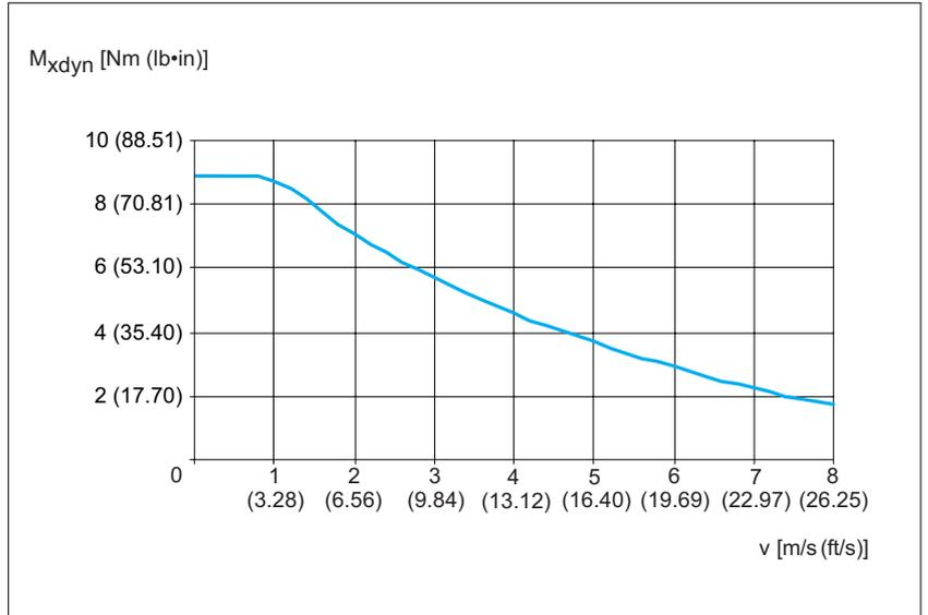
Figure 22: PAS42BR Maximum torque carriage  $M_{xdyn}$
