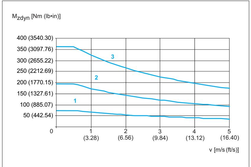
Figure 33: PAS42BB Maximum torque carriage  $M_{zdyn}$
