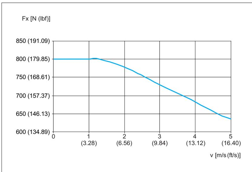
Figure 27: PAS42BB Maximum feed force  $F_x$
