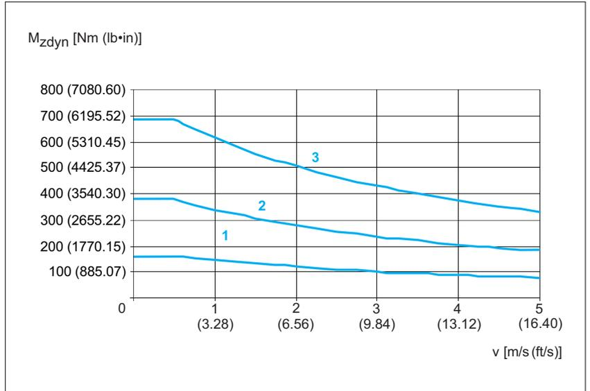
Figure 44: PAS43BR Maximum torque carriage  $M_{zdyn}$
