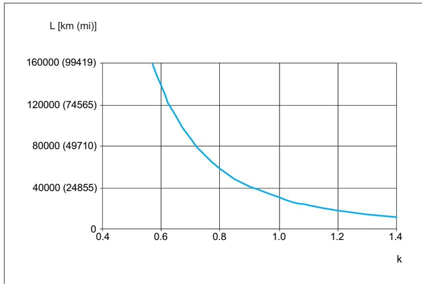
Figure 25: PAS42BR Service life load curve
