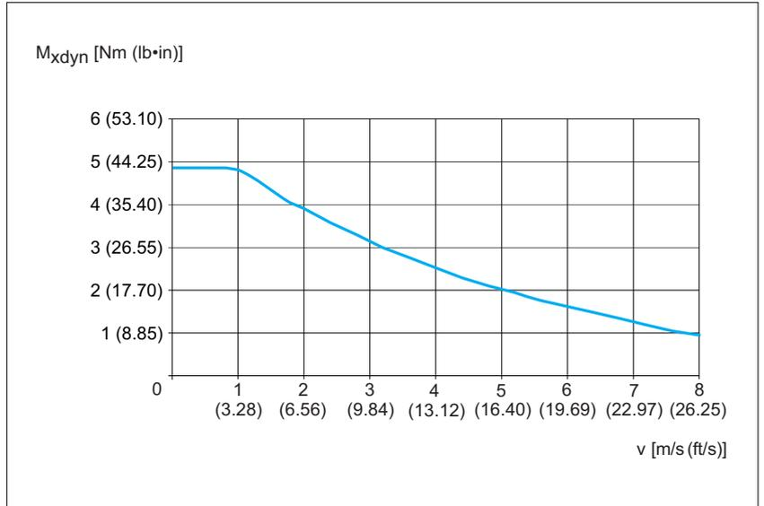
Figure 11: PAS41BR Maximum torque carriage  $M_{xdyn}$
