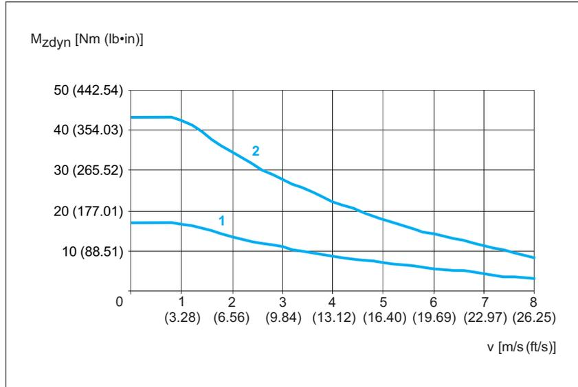
Figure 13: PAS41BR Maximum torque carriage  $M_{zdyn}$
