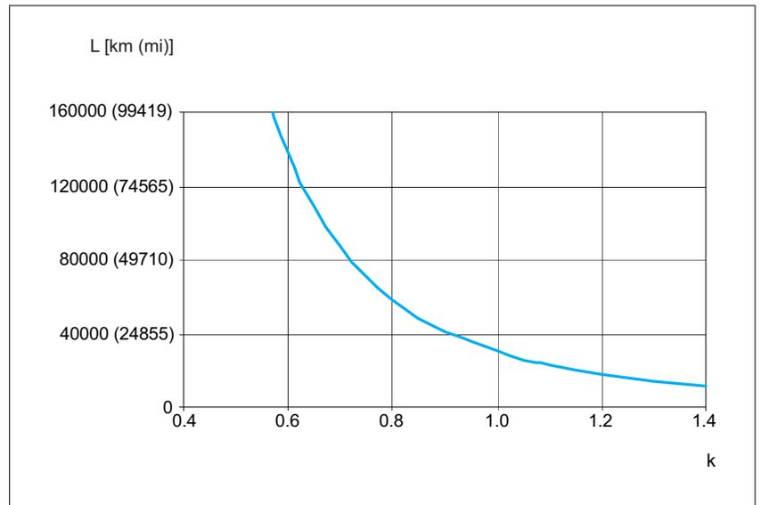
Figure 34: PAS42BB Service life load curve
