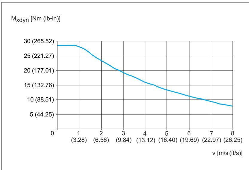
Figure 42: PAS43BR Maximum torque carriage  $M_{xdyn}$
