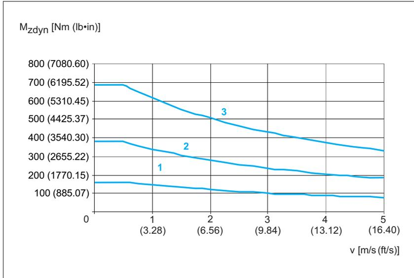
Figure 53: PAS43BB Maximum torque carriage  $M_{zdyn}$
