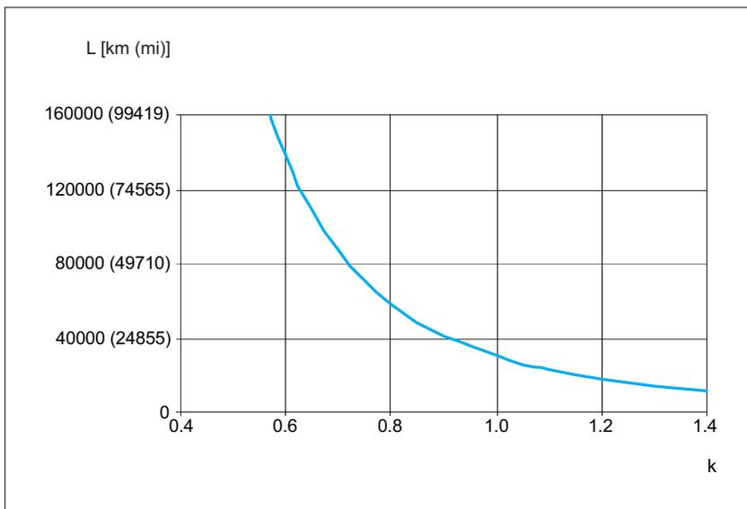
Figure 65: PAS44BB Service life load curve
