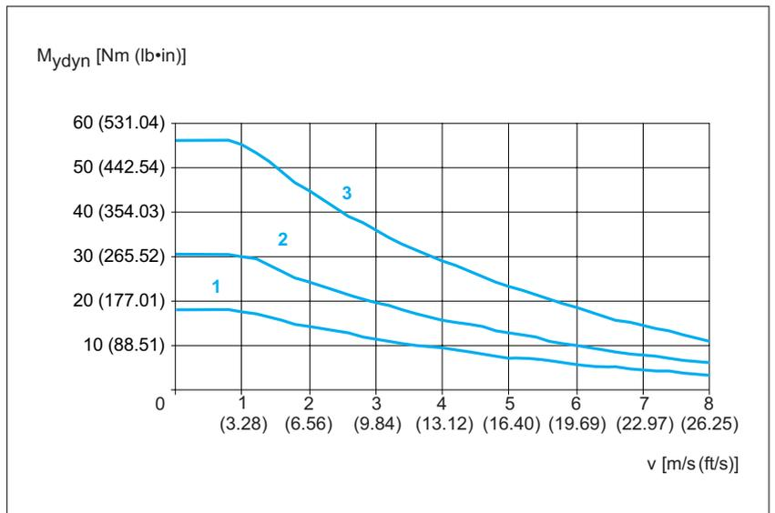
Figure 23: PAS42BR Maximum torque carriage  $M_{ydyn}$
