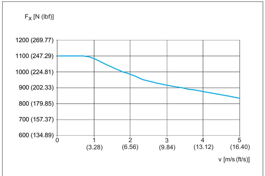
Figure 47: PAS43BB Maximum feed force  $F_x$
