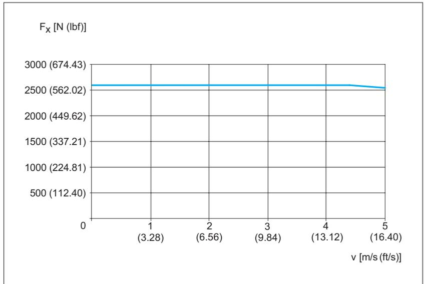
Figure 58: PAS44BB Maximum feed force  $F_x$
