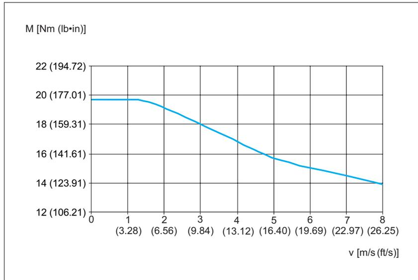
Figure 21: PAS42BR Maximum driving torque  $M_{max}$
