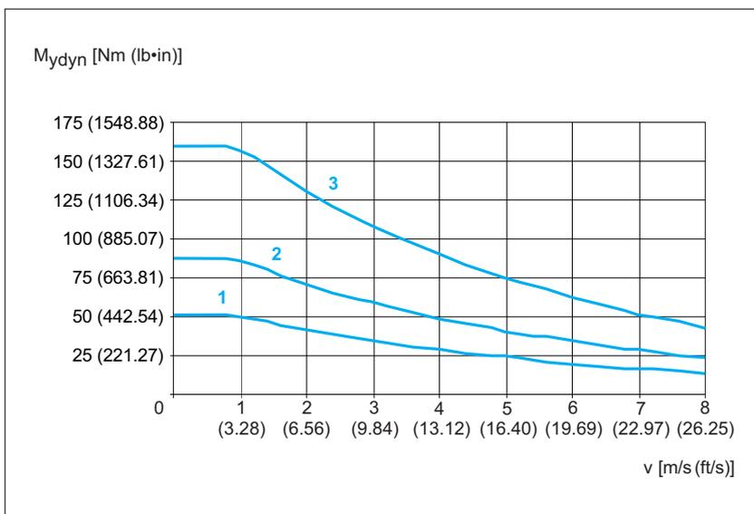
Figure 43: PAS43BR Maximum torque carriage  $M_{ydyn}$
