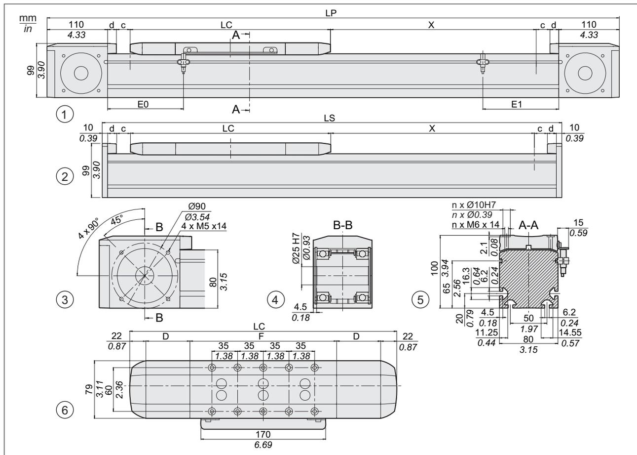
Figure 56: Dimensional drawings PAS43B
