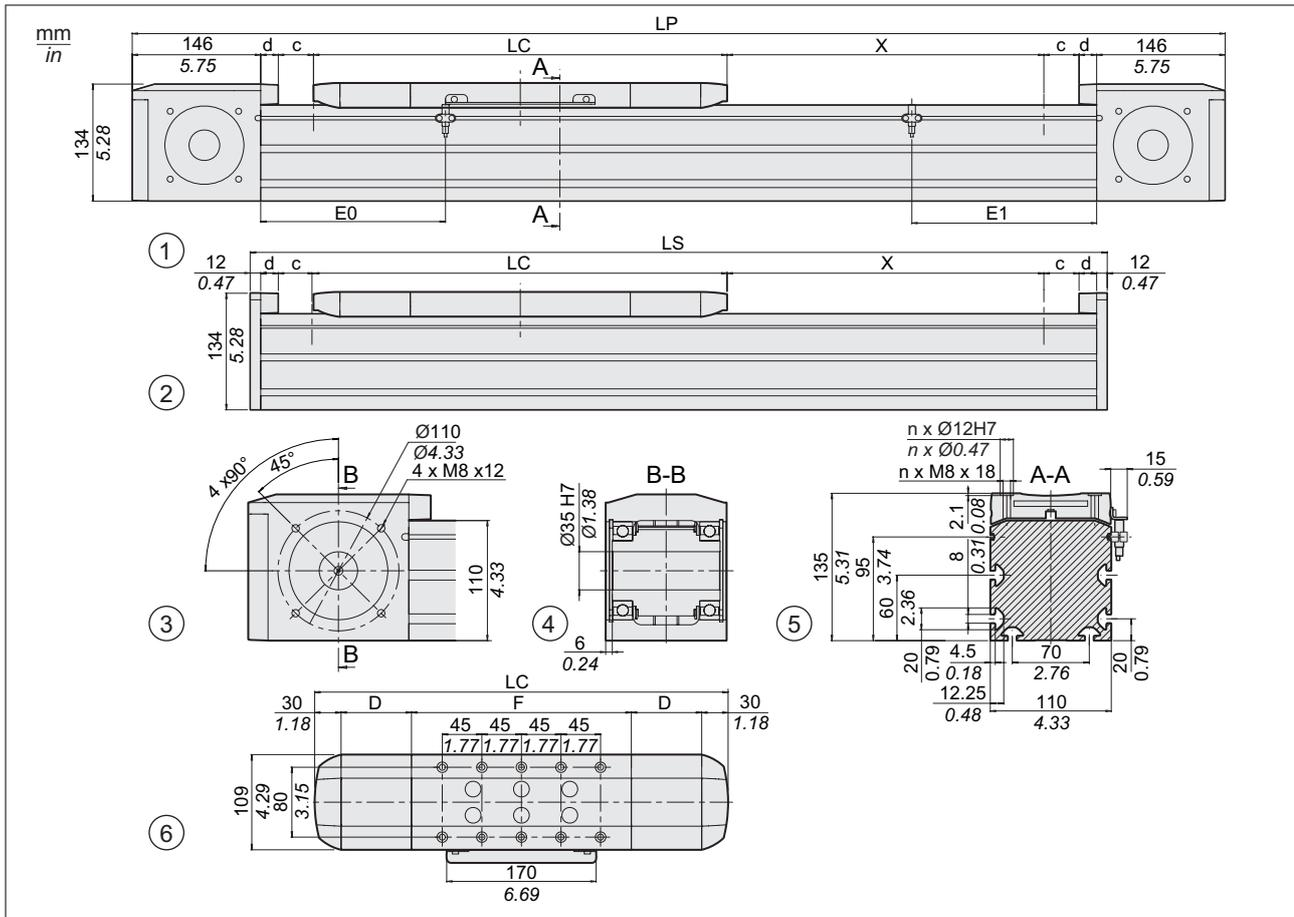
Figure 67: Dimensional drawings PAS44BB
