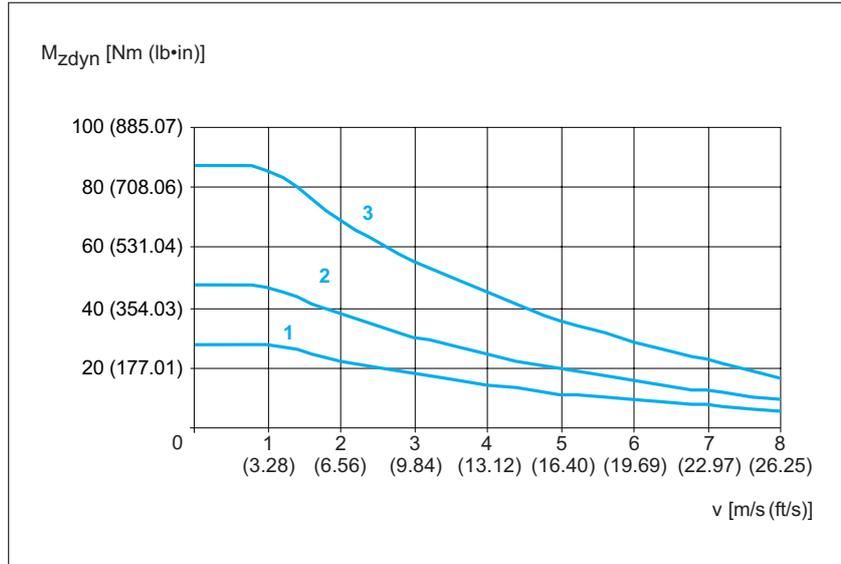
Figure 24: PAS42BR Maximum torque carriage  $M_{zdyn}$
