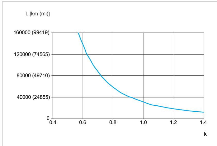
Figure 14: PAS41BR Service life load curve
