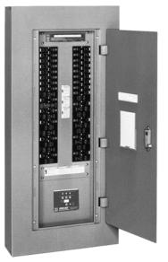
The Surgelogic<sup>®</sup> IMA series surge protective device (SPD) is a modular parallel transient voltage surge suppressor (TVSS). The IMA device is a multi-stage suppression circuit consisting of field-proven, fast-acting, 34 mm metal oxide varistors (MOVs).
