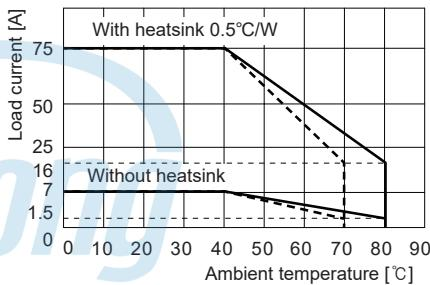
⚠ Since effectiveness of the heat radiation is decreased when multiple SSRs are installed closely, please supply less than 50% of the rated load current.
