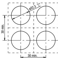
When mounting 100/110V AC, 200/220V AC, 110V DC units on 30mm centers vertically and horizontally, keep the ambient temperature below 40°C.
