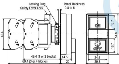
Flush (top), Flush (bottom) (380V AC minimum)
