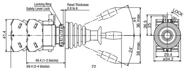
Terminal Screws M3.5 Integrated Terminal Cover
