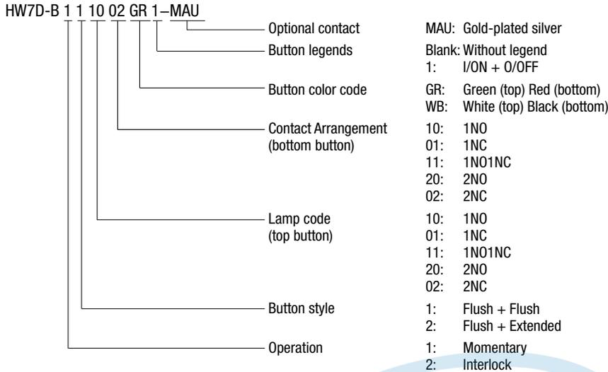
Dual Pushbutton Switches [with pilot light] (Page 21)
