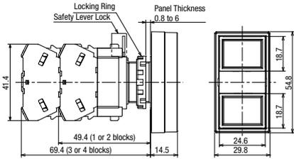
**With Pilot Light** Terminal screws: M3.5, integrated terminal cover
