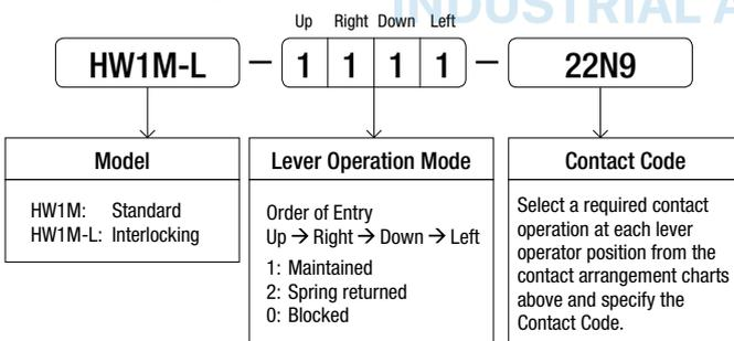
Contact Block Mounting Position and Lever Operation Position
