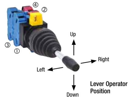
• The lever operator of the interlocking type HW1M-L is locked only in the center position. Pull on the interlocking lever before operating the lever up/down/right/left.
