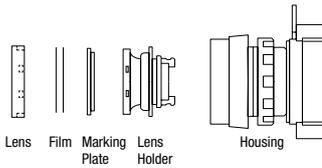
Note: Films are not supplied. When inserting a film, make sure that the marking plate is installed with its uneven side facing the lens holder.
