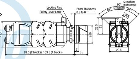
**Illuminated Selector Switch (Lever Operator)**
