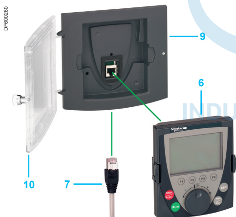
Remote location of the graphic display terminal on enclosure door: 6 + 7 + 9 if IP 54, 6 + 7 + 9 + 10 if IP 65
