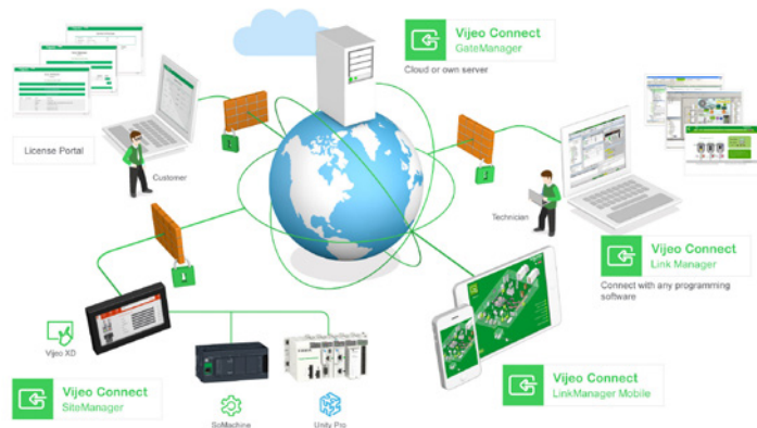
Vijeo Connect for remote programming access to the HMI and its connected devices
