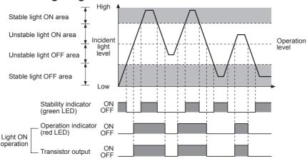
\*\*The waveforms of "Operation indicator" and "Transistor output" are for Light ON operation. They are opposite operation for Dark ON operation.
