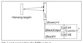
X1: Load connection for NPN output **%2: Load connection for PNP output**
