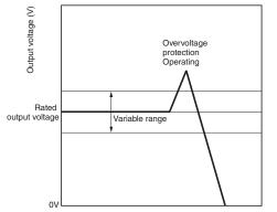
Note: Do not turn ON the power again until the cause of the overvoltage has been removed.
