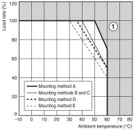
**Open-frame Models and Models with Chassis: 100W**
