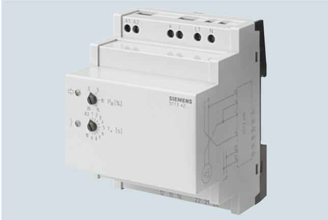
The 5TT3424 and 5TT3425 reverse power relays monitor the direction of the energy transport in an electric grid. This may be necessary where public grids and industrial grids intersect, e.g. when using emergency generators, motor-driven generators, etc.
