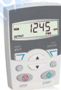
Basic control panel
