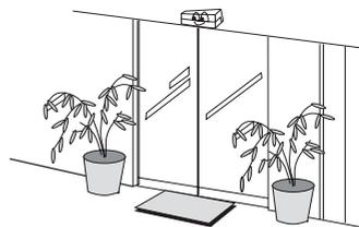
5. The sensing lens must be installed face to the door's threshold. If it faces the wall or roof, it may not operate normally.
