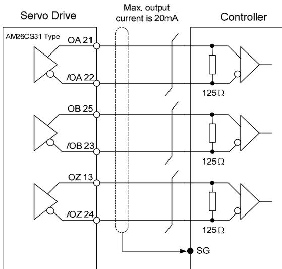
**C14: Encoder output signal (Photocoupler)**
