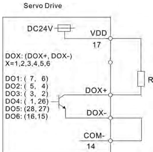
**C6:** Wiring of DO signal, for the use of internal power supply, inductive load
