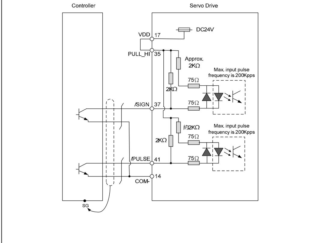
**C3-2:** The source of pulse input is open-collector PNP equipment which applies the internal power of the servo drive.
