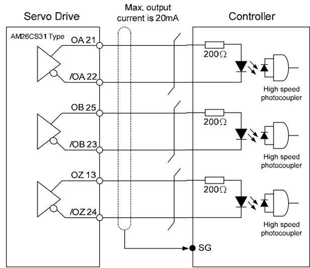
**C15: Encoder OCZ output (Open-collector Z-pulse output)**
