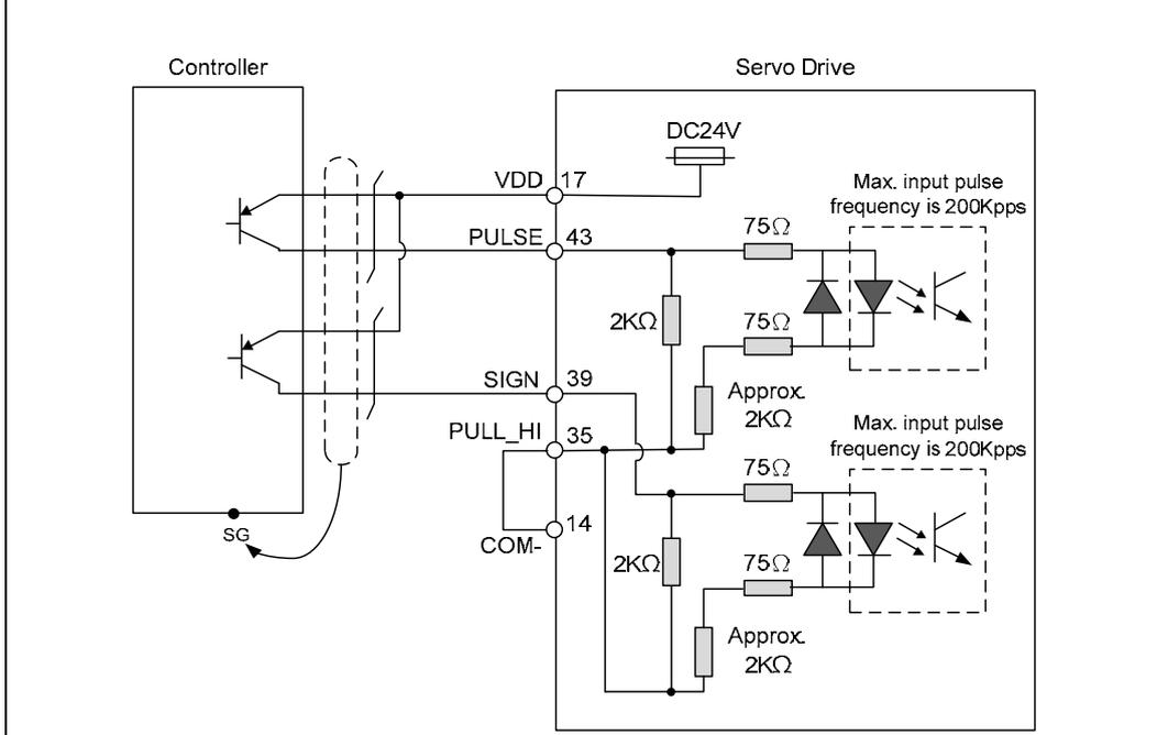
**C3-3:** The source of pulse input is open-collector NPN equipment which applies the external power of the servo drive.
