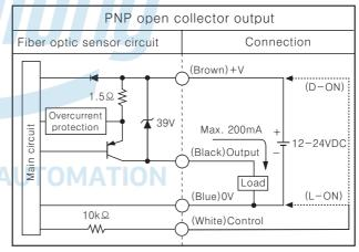
\*\*When select Dark ON or Light ON, please use control wire(White) Light ON: Connect control wire to 0V Dark ON: Connect control wire to +V
