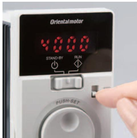
The rotation direction of the motor can be changed easily
