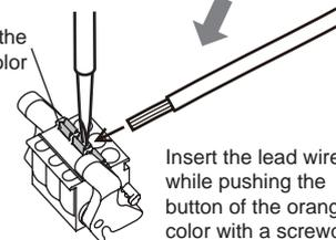
Insert the lead wire while pushing the button of the orange color with a screwdriver.
