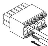
Crimp terminals can also be used to connect.
