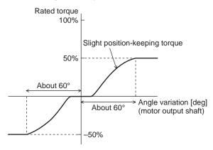
Slight position-keeping torque characteristic
