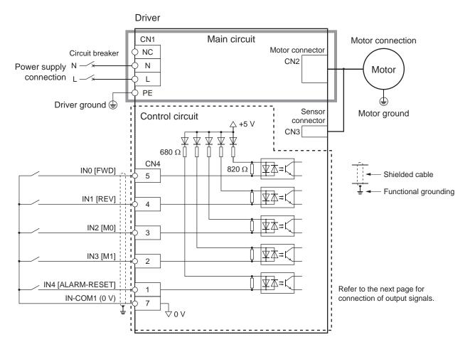
The I/O signal in the brackets [] is the assignment at the time of shipment.
