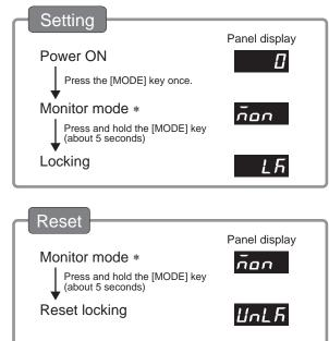
If the setting value of the operation data or parameter is tried to change, "LF" is displayed for about one second.
