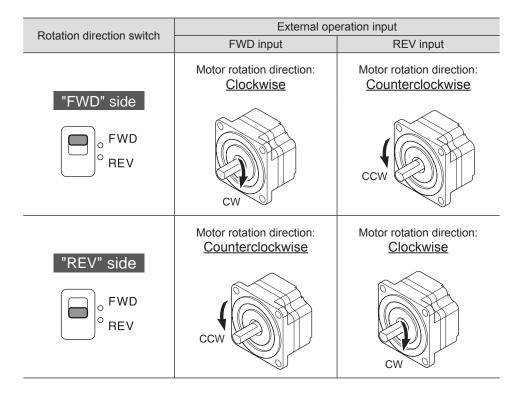
If the rotation direction switch is changed, the motor will decelerate to a stop and start rotating in the direction being switched.
