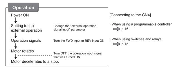
This operation example is for when the rotation speed is set to the operation data No.0.
