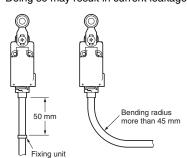
When wiring, be sure to prevent penetration of a liquid such as water or oil through the cable end.
