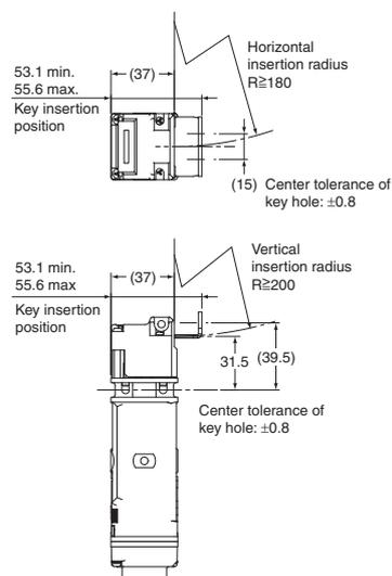
With Top-inserted Operation Key
