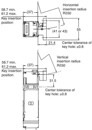
**With Top-inserted Operation Key**
