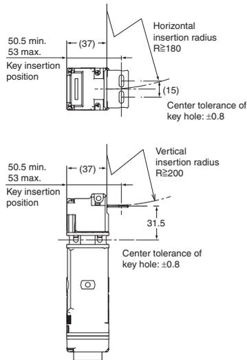
With Top-inserted Operation Key
