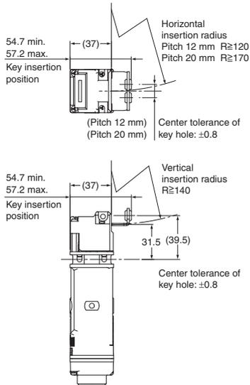
**With Top-inserted Operation Key**
