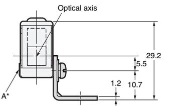
\*The Mounting Bracket can be attached to side A.
