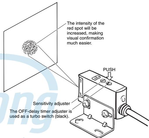
**Using the E39-R5 Optical Axis Reflector for Through-beam Sensors**
