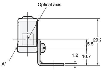
\*The Mounting Bracket can be attached to side A.
