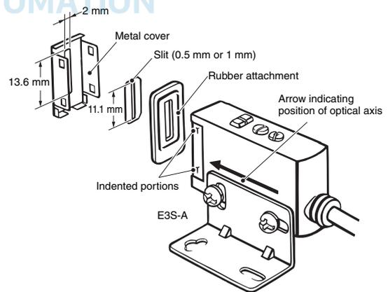
Apply the Slit to the lens of the Photoelectric Sensor marked with an arrow indicating the position of the optical axis (apply it to the bottom lens of Horizontal Sensors and the top lens of Vertical Sensors).
