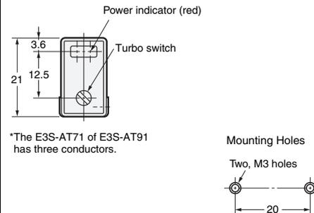
Note: Models numbers for Through-beam Sensors (E3S-AT□1) are for sets that include both the Emitter and Receiver.
