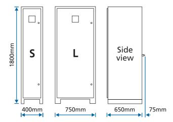
Overall depth of 725mm is required to allow a ventilation gap of 75mm (rubber back-stop provided ensures this distance is maintained)
