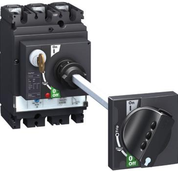
EasyPact EZS with an extended rotary handle installed at the back of a switchboard, with the keylock option and key.
