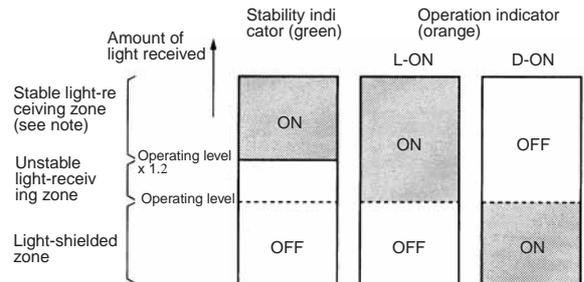
Note: If the Receiver is set to the stable light-receiving zone, it will become more resistant to environmental fluctuations such as temperature, voltage, dust, and setting deviation after installation. For applications where a stable light-receiving zone is not obtained, attention must be paid to environmental fluctuations.
