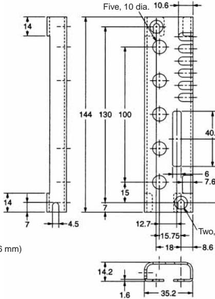
Material: Steel (Thickness: 1.6 mm)
