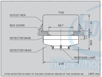
\*\*NOTE : Cleaning of the detector head can be easily done after removing the labyrinth cover.
