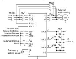
Electronic bypass sequence connection diagram (standard model)
