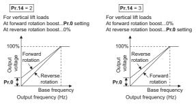
Switching applied load selection with a terminal (setting value "4,
