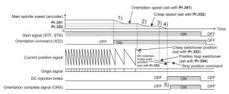
Using the FR-A8TP (motor end) together with the plug-in option FR-A8AP/FR-A8AL/FR-A8APR (machine end) enables machine end orientation control.
