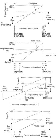
Analog input display unit changing (Pr.241) The analog input display unit (%/V/mA) for analog input bias and gain calibration can be changed.
