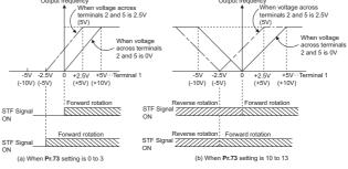
Terminal 1 (frequency setting auxiliary input) is added to terminal 2 or 4 main speed setting signal.
