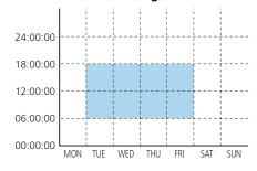
Operation schedule can be set according to actual condition by using four timers.
