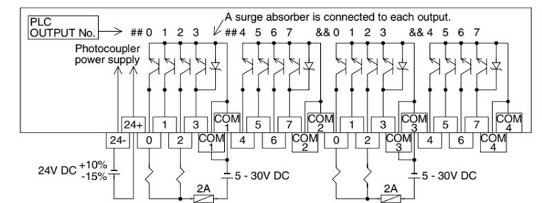
Terminal blocks are not equipped with built-in fuses. In order to prevent breakdown of circuits caused by load short-circuit, provide a fuse of 2 A for every four points.
