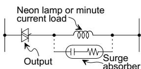
To a neon lamp or a minute current load of 0.4VA/100V AC, 1.6VA/200V AC or less, connect a surge absorber in parallel.
