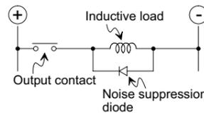
Connect a noise suppression diode to a DC inductive load in parallel. If the diode is not connected, the life time of the contact becomes considerably shorter. Select a noise suppression diode whose reverse withstand voltage is 5 to 10 times or more the load voltage and whose current in the forward direction is not less than the load current.
