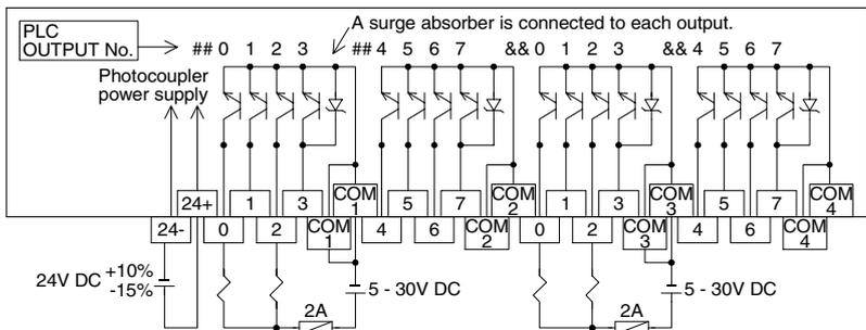
Terminal blocks are not equipped with built-in fuses. In order to prevent breakdown of circuits caused by load short-circuit, provide a fuse of 2 A for every four points.
