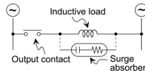
When a surge absorber is connected to an AC inductive load in parallel, noise generation is reduced.
