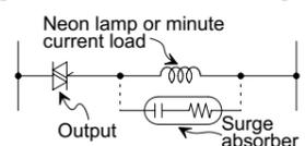
To a neon lamp or a minute current load of 0.4VA/100V AC, 1.6VA/200V AC or less, connect a surge absorber in parallel.
