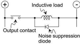
Connect a noise suppression diode to a DC inductive load in parallel. If the diode is not connected, the life time of the contact becomes considerably shorter.
