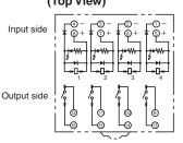
**Note1**: Make sure that the polarity of the input terminal is correct
