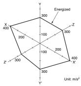
Sample: G6B-1114P-US Number of Relays: 12 pcs Test Conditions: Shock is applied in  $\pm X$ ,  $\pm Y$ , and  $\pm Z$  directions three times each with without
