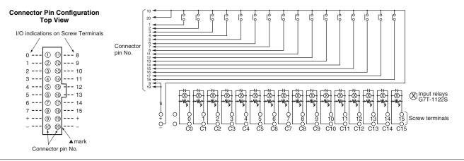
Note: Pin numbers are indicated for convenience. The ▲ mark can be used to determine orientation.
