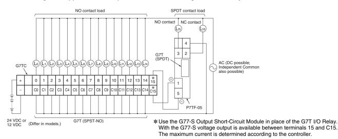
**Note:** If more than one G77-S Output Short-Circuit Module is employed, the voltage output of the terminals on the G7TC is as follows: G7TC-OC16: The positive side (the lower row) connects to the common line internally. G7TC-OC16-1: The negative side (the upper row) connects to the common line internally.
