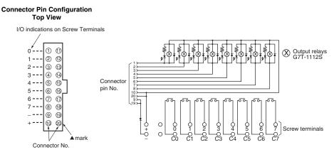
Note: Pin numbers are indicated for convenience. The **A** mark can be used to determine orientation.
