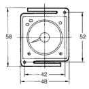
Note: The mounting panel thickness should be 1 to 5 mm.
