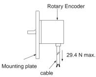
Do not pull the cable of the E6B2-C rotary Encoder after the E6B2-C Rotary Encoder is mounted to a panel. Do not apply any shock to the hollow shaft or the body.
