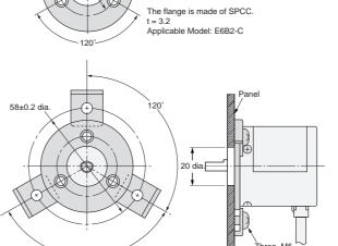
Three, 3.5-dia. holes with 6.5 dia. countersunk holes
