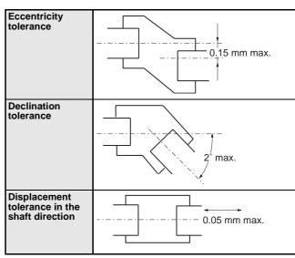
If the eccentricity or declination value exceeds the tolerance, an excessive load imposed on the shaft may damage the Rotary Encoder or shorten the life of the Rotary Encoder.
