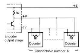
E: Voltage supplied to Rotary Encoder
