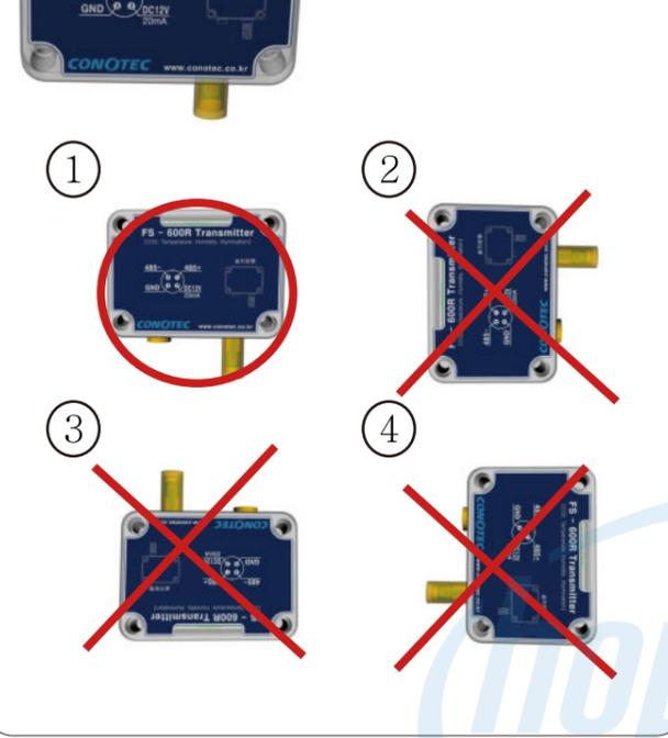
1. FS-600R must be installed in the same direction as O mark (No. 1).
