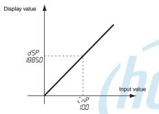
When displaying a flowrate (e.g., in  $\mathscr{U}$ min or  $\mathscr{U}$ h), make the scaling settings after confirming the I/O characteristics of the flowrate sensor. There are flowrate sensors that output analog signals. If this kind of flowrate sensor is used, consider using the K3MA-J.
