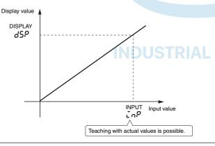
Instead of setting by inputting with the riangle Up Key and riangle Shift Key, current values can be input as scaling input values for teaching. This is useful for making settings while checking the operation status of the K3MA-F.
