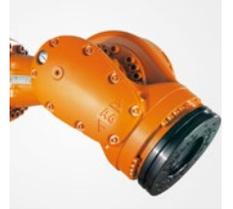
**1** Robot knee positioned lower and further forward for greater downward reach
