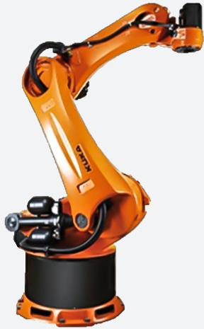
This powerful palletizing robot, the KUKA KR 470-2 PA, is just what your production line needs. It can handle up to 470 kg with a reach of 3150 mm, and is paired with the KR C4 controller. The KR 470-2 PA also brings your floor more space and simplified integration as it offers a compact design and low weight and fastening elements.
