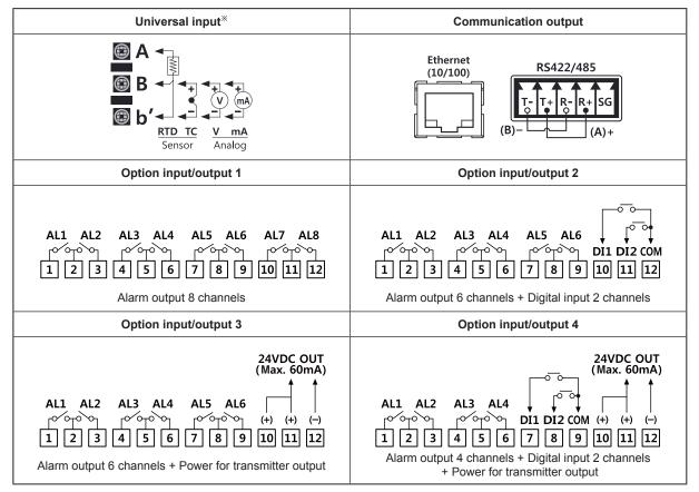
$\times$  In case of current input, connect 250 $\Omega$  resistance at external part.
