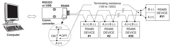
XIt is recommended to use Autonics communication converter; SCM-US48I (USB to RS485 converter, sold separately),
