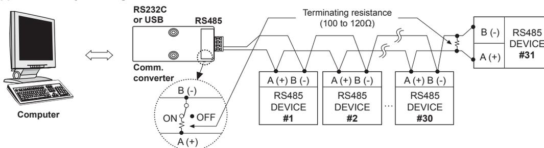
※It is recommended to use Autonics communication converter; SCM-US48I (USB to RS485 converter, sold separately), SCM-38I (RS232C to RS485 converter, sold separately). Please use twisted pair wire for RS485 communication.
