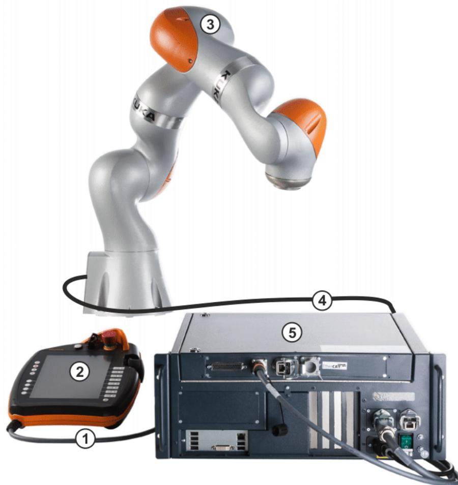
**Fig. 3-1: Overview of robot system**
