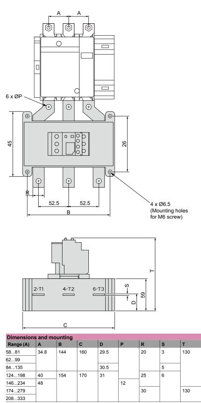
The LRE48 $\bullet$  is mounted separatly from the contactor (LCE120...300) on a mounting plate with 4 x M6 screws (torque = 6 N.m).
