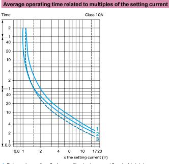
Balanced operation, 3-phase, without prior current flow (cold state).
