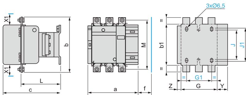
X1 (mm) = minimum electrical clearance according to operating voltage and breaking capacity.
