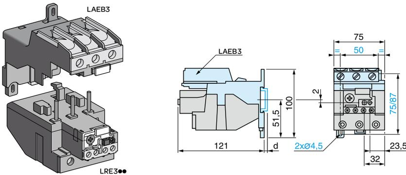
Mounting on DIN rail AM1D
