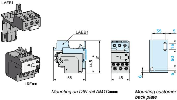
Mounting on DIN rail AM1D
