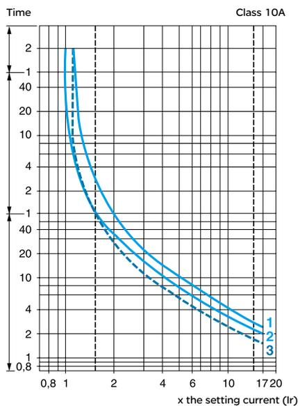
1. *Balanced operation, 3-phase, without prior current flow (cold state).*
