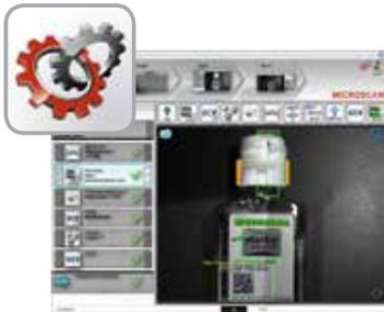
AutoVISION is the easiest software available for basic to mid-range vision applications. Its intuitive interface guides the user to connect to a device, configure the hardware, program the job and monitor results. Jobs are fully scalable across cameras, software, industrial systems, PCs and mobile devices.
