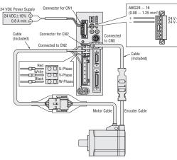
♦ Connecting the Electromagnetic Brake Connect 24 VDC.
