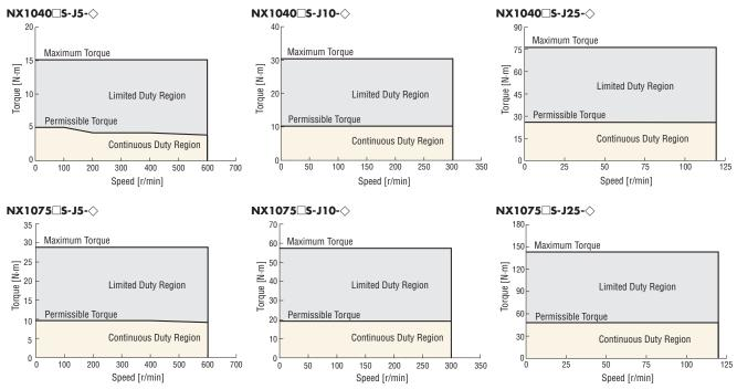
Either A (standard) or M (electromagnetic brake type) indicating the motor shaft configuration is entered where the box □ is located within the product name. A number indicating the desired length of 1 (1 m), 2 (2 m) or 3 (3 m) for the cables included with the product is entered where the box ◇ is located within the product name.
