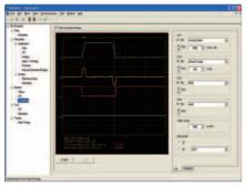
\*Monitoring the operating status waveform requires the data setting software (MEXEO2), which is sold separately.
