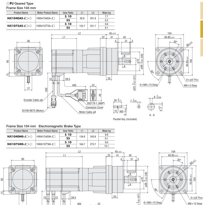
400 22 27 400 00 ≘ Encoder Cable  $\phi 6$ M 30-0.21 7-0.09 350779-1 (AMP) ٩́Π Connector Cover 55100-0670 (Molex) Motor Cable  $\phi 8$ 15 \<u>M3</u> 19 Cable for Electromagnetic Brake  $\phi 6$ A-A 5557-02R-210 (Molex) 18.5 Connector Cover Parallel Key (Included)
