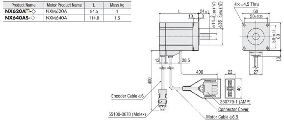
•Either A (single-phase 100-115 VAC) or C (single-phase 200-230 VAC/three-phase 200-230 VAC) indicating the power supply voltage is entered where the box is located within the product name. A number indicating the desired length of 1 (1 m), 2 (2 m) or 3 (3 m) for the cables included with the product is entered where the box is located within the product name.
