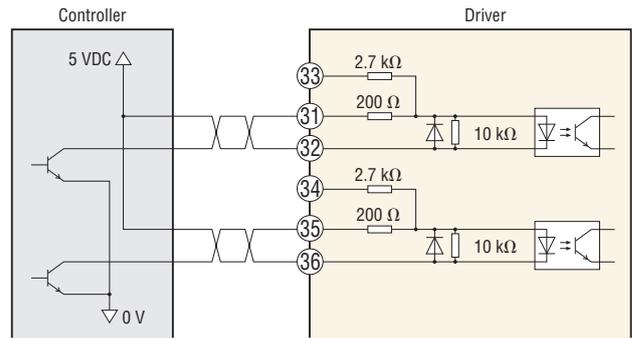
When the input voltage is 24 VDC
