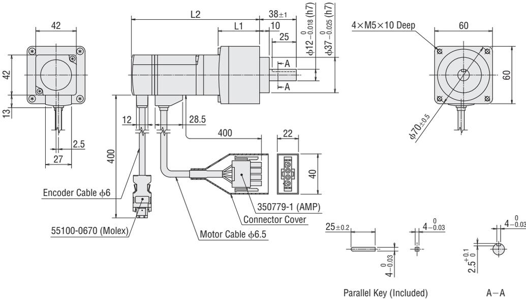
Frame Size 60 mm Electromagnetic Brake Type
