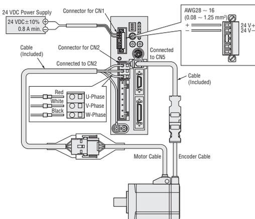
◇ Connecting the Electromagnetic Brake
