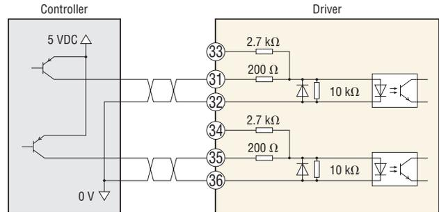
When the input voltage is 24 VDC
