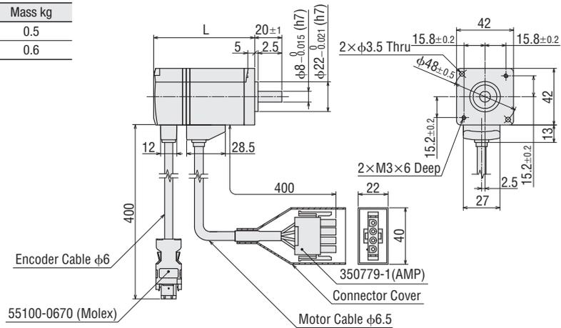
Frame Size 42 mm Electromagnetic Brake Type
