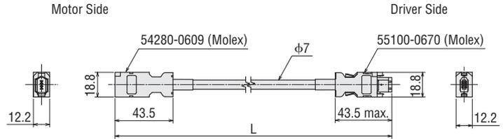
● Cables for Electromagnetic Brake (Electromagnetic brake type only)
