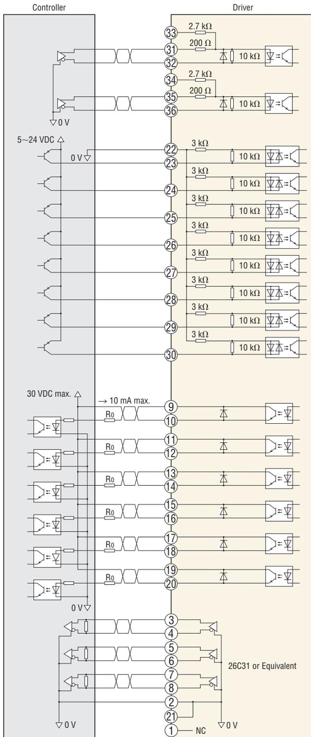
When the input voltage is 5 VDC
