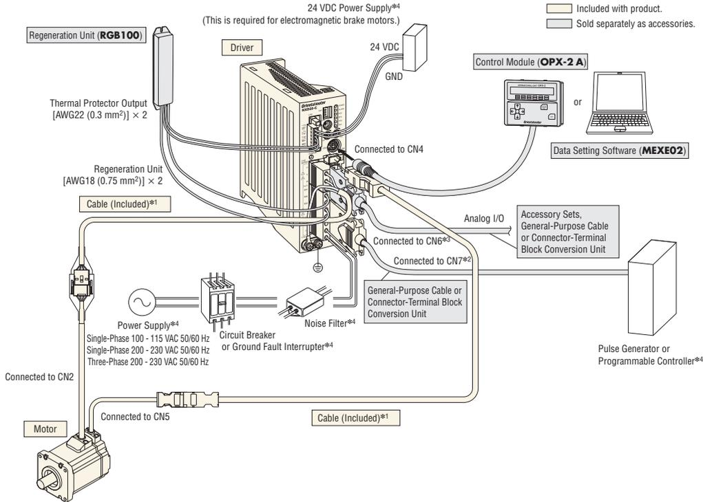
\*1 1 m, 2 m or 3 m cables are included with the product. If you need cables longer than 3 m or flexible cables, select appropriate cables from the accessories (sold separately).
