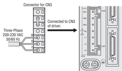
◇ Connecting the Control Power Supply
