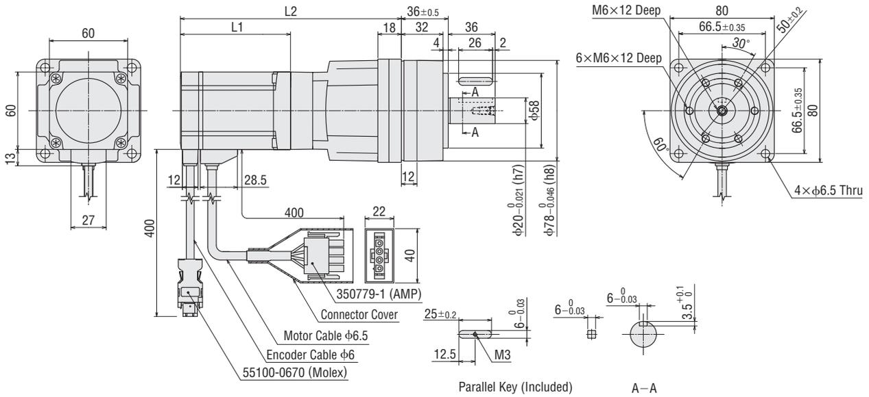
Frame Size 80 mm Electromagnetic Brake Type
