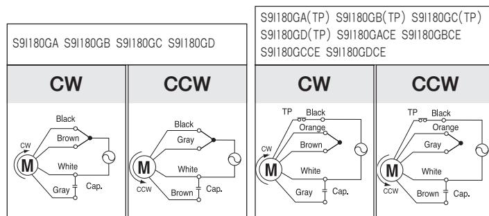
Change the direction of motor rotation only after the motor stops completely. If an attempt is made to change the direction of rotation while the motor is running, the motor may ignore the reversing command or change its direction of rotation after some delay.
