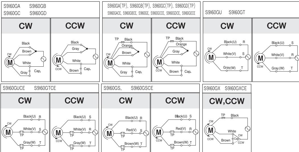
Change the direction of motor rotation only after the motor stops completely. If an attempt is made to change the direction of rotation while the motor is running, the motor may ignore the reversing command or change its direction of rotation after some delay.
