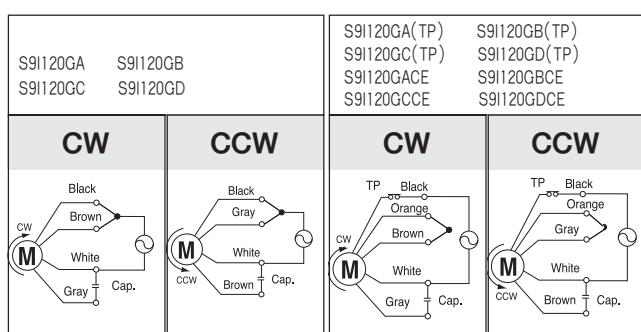
Change the direction of motor rotation only after the motor stops completely. If an attempt is made to change the direction of rotation while the motor is running, the motor may ignore the reversing command or change its direction of rotation after some delay.
