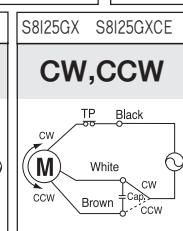
Change the direction of motor rotation only after the motor stops completely. If an attempt is made to change the direction of rotation while the motor is running, the motor may ignore the reversing command or change its direction of rotation after some delay.
