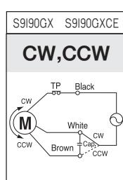
Change the direction of motor rotation only after the motor stops completely. If an attempt is made to change the direction of rotation while the motor is running, the motor may ignore the reversing command or change its direction of rotation after some delay.
