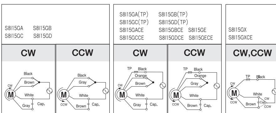
Change the direction of motor rotation only after the motor stops completely. If an attempt is made to change the direction of rotation while the motor is running, the motor may ignore the reversing command or change its direction of rotation after some delay.
