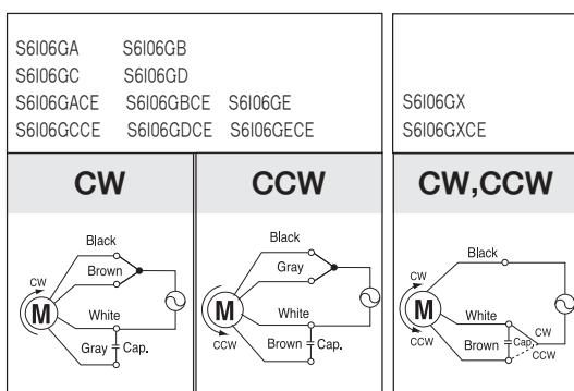
Change the direction of motor rotation only after the motor stops completely. If an attempt is made to change the direction of rotation while the motor is running, the motor may ignore the reversing command or change its direction of rotation after some delay.
