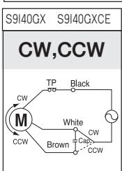
Change the direction of motor rotation only after the motor stops completely. If an attempt is made to change the direction of rotation while the motor is running, the motor may ignore the reversing command or change its direction of rotation after some delay.
