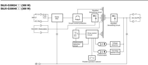
Note: Short-circuit the input voltage selector terminals if the input is 100 to 120 VAC. Keep the terminals open if the input is 200 to 240 VAC.
