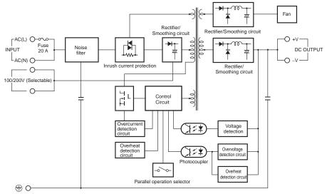
**Note:** Short-circuit the input voltage selector terminals if the input is 100 to 120 VAC. Keep the terminals open if the input is 200 to 240 VAC.
