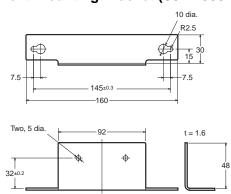
**Note:** Mounting Brackets are provided in a set, one for the right side and one for the left side.
