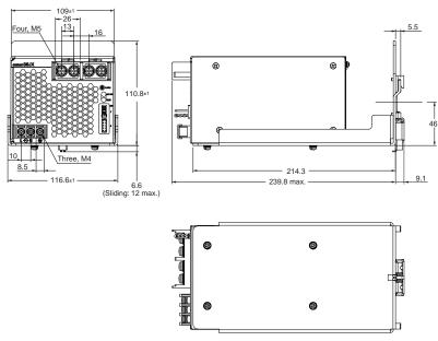
Note: Use a metal DIN Rail when mounting a 600-W model to a DIN Rail.
