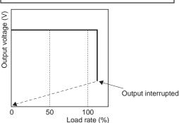
If an excessive current flows for 5 s or more, the output will be turned OFF and simultaneously the protection-ON alarm indicator will be lit. To reset the S8JX, turn OFF the power, leave the S8JX for at least three minutes, and then turn it ON again.
