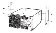
**Note:** To provide ventilation space, the body will shift forward by 23.6 mm from the mounting surface.
