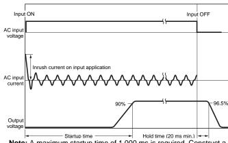
**Note:** A maximum startup time of 1,000 ms is required. Construct a system configuration that considers the startup time of other devices.
