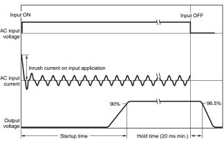
Note: A maximum startup time of 500 ms is required (650 ms for 300 W). Construct a system configuration that considers the startup time of other devices.
