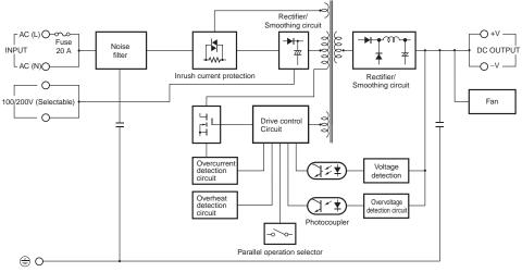
Note: Short-circuit the input voltage selector terminals if the input is 100 to 120 VAC. Keep the terminals open if the input is 200 to 240 VAC.
