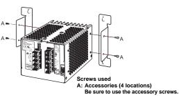
Note: For ventilation of the back surface, the body should be placed 21.6 mm in front of the mounting side.
