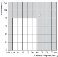
Note: 1. Internal parts may occasionally deteriorate or be damaged. Do not use the Power Supply in areas outside the derating curve (i.e., the area shown by shading ① in the above graph).
