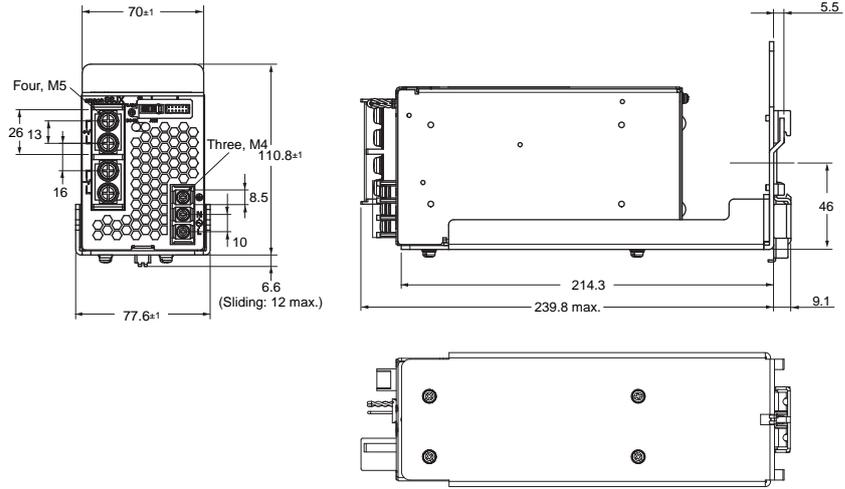
**Note:** Use a metal DIN Rail when mounting a 300-W model to a DIN Rail.
