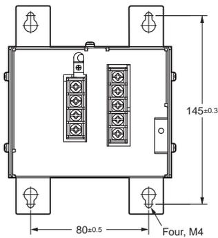
**Attaching the Mounting Brackets**
