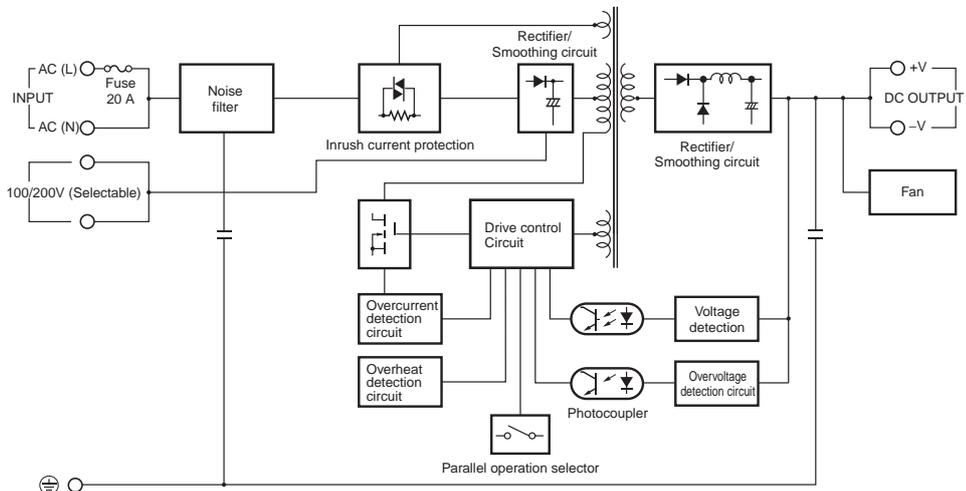
**Note:** Short-circuit the input voltage selector terminals if the input is 100 to 120 VAC.
