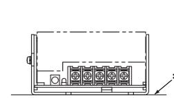
**Note:** 1. Improper mounting will interfere with heat dissipation and may occasionally result in deterioration or damage of internal parts. Use the standard mounting method only.
