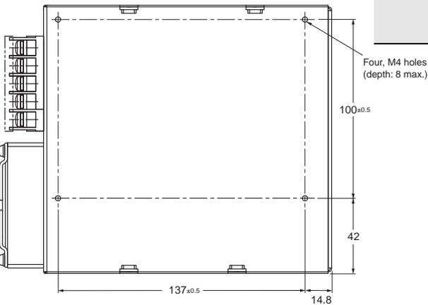
**Mounting Bracket Provided with Front-mounting Power Supplies (A)**
