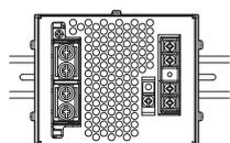
**Note:** 1. Improper mounting will interfere with heat dissipation and may occasionally result in deterioration or damage of internal parts. Use the standard mounting method only.
