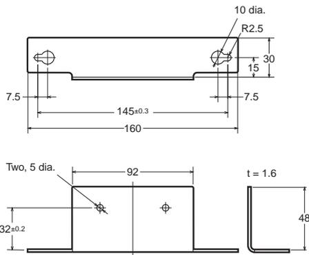
**Note:** Mounting Brackets are provided in a set, one for the right side and one for the left side.
