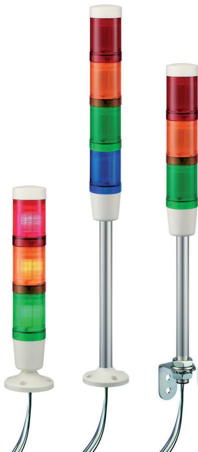
XVM Tower lights supplied pre-assembled and pre-cabled, with 1, 2, 3 or 4 illuminated units, each one fitted with a buzzer and a fixing base
