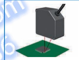
Inspecting for Board Coplanarity
